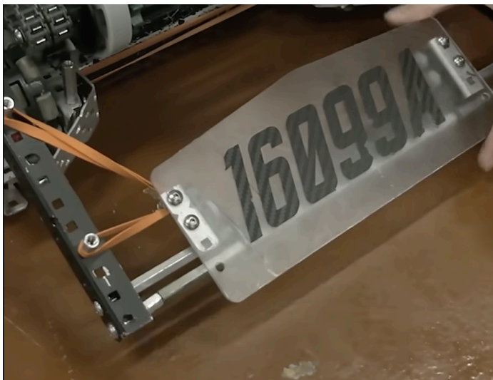
Matchloading Mechanism Regular Position (16099A Pits & Parts Interview)
