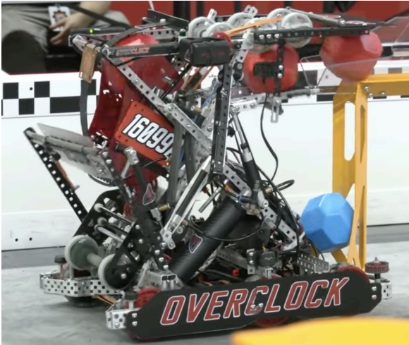
S-Shaped Intake (Pits and Parts Interview with 16099A)
